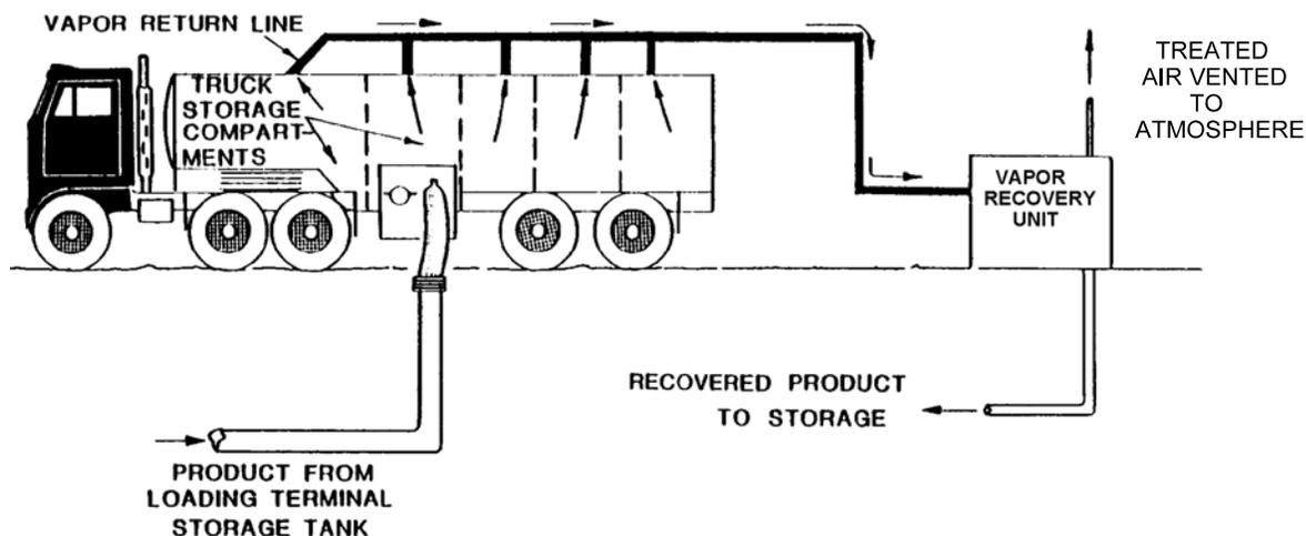
Figure 5.2-6. Tank truck loading with vapor recovery.
